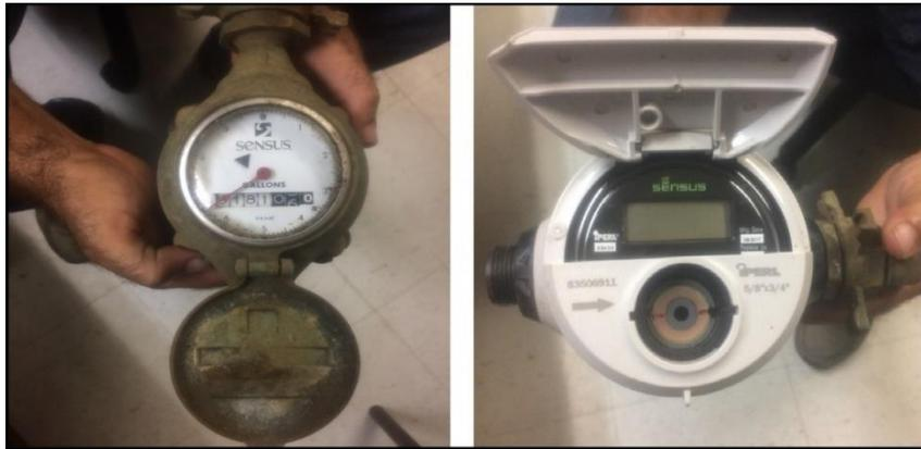
Figure 10: Water meters currently used by ASPA showing (a) (left) older type mechanical totalizing magnetic drive meters that must be read manually, and (b) (right) digital electromagnetic meter with wireless data transmission capabilities.
