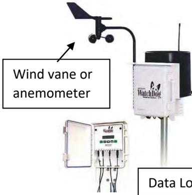
Wind vane or anemometer
