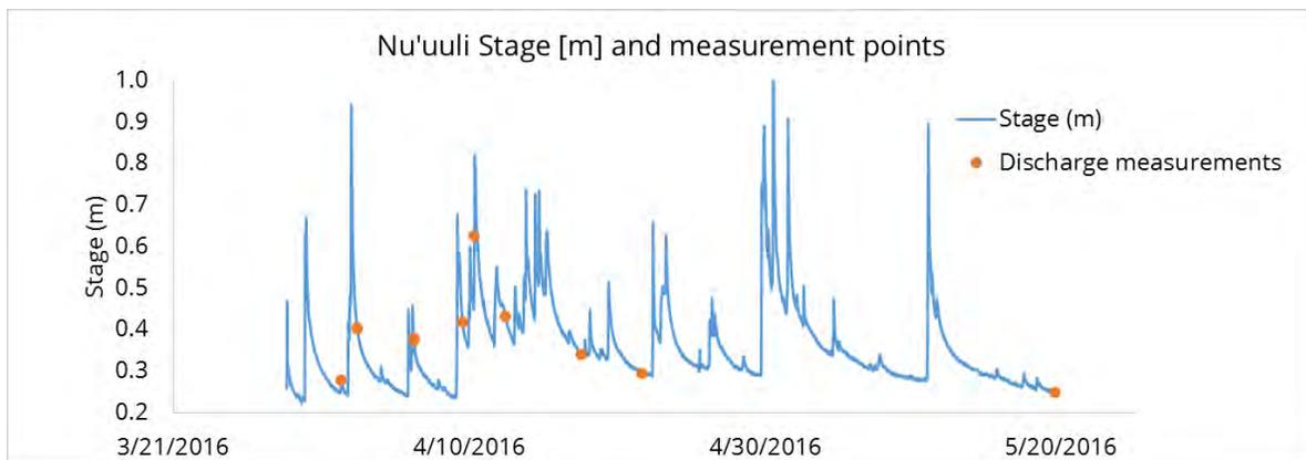
Figure 5. Example of stream stage and times where streamflow measurements were taken.
