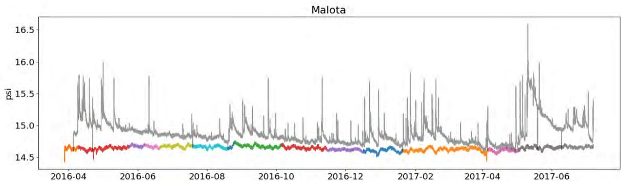
Figure 4. Example plot of raw stream stage data (grey line) and barometric pressure data (colored lines) from a barometer located at ASPA HQ. The barometric pressure data is subtracted from the stage data to obtain height of the water column above the PT.
