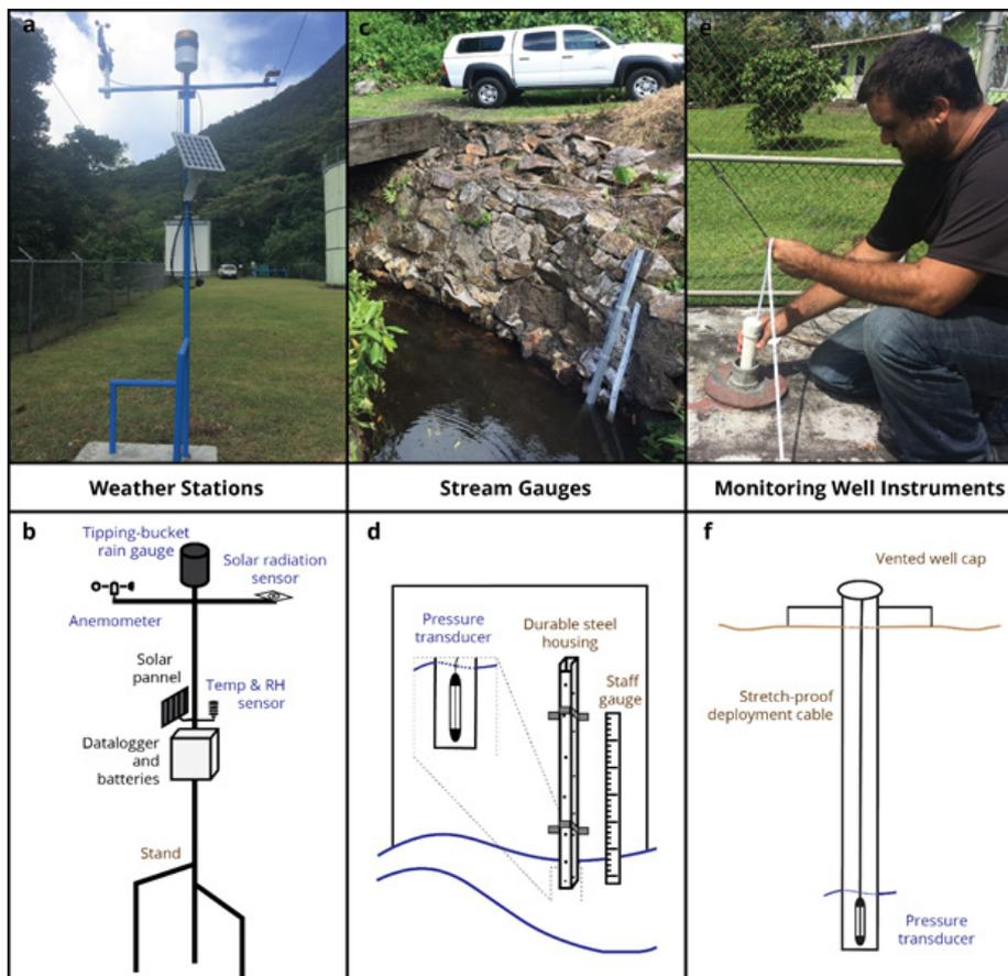
Figure 2: Examples of ASPA-UHWRRC weather station, stream gauge, and monitoring well network instruments with schematics. Blue text on schematics indicates sensors and brown text indicates hardware and infrastructure.
