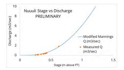
Figure 6. Example stage-discharge rating curve relationship based on modified Manning's discharge calculation
