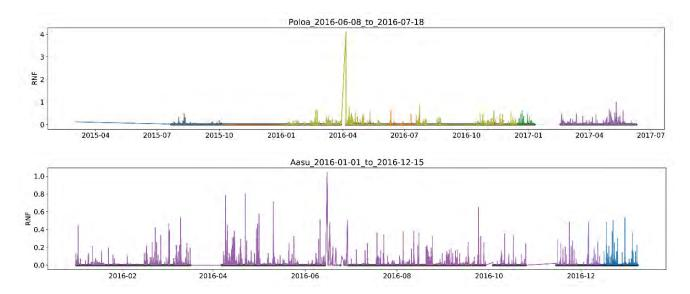
Figure 2. Example plots of concatenated rainfall data series. Note gaps in datasets due to instrument malfunction.
