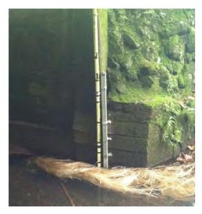
and the gauging pool is fairly deep (about 40 cm at low water). The level control currently consists of a rock bar and is subject to being moved in a flood. Data consistency at this site would be improved by installation of a weir. Both high- and low-flow discharge measurements have been taken underneath or just downstream of the bridge.
