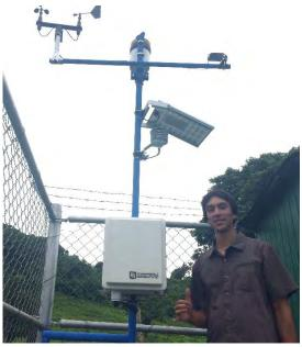
station is now mounted at the same location on a three legged free standing support tower that is bolted to the concrete slab below. The SR meter, anemometer, and rain gauge are located at a height of 3 m above ground surface and temperature and RH sensors are mounted at 2 m above the ground. Access to well 128 is off of a paved concrete road accessed via a right turn within the village of Aasu while at the top of the main Aoloau Road.
