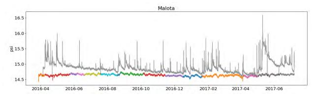
Figure 4. Example plot of raw stream stage data (grey line) and barometric pressure data (colored lines) from a barometer located at ASPA HQ. The barometric pressure data is subtracted from the stage data to obtain height of the water column above the PT.
