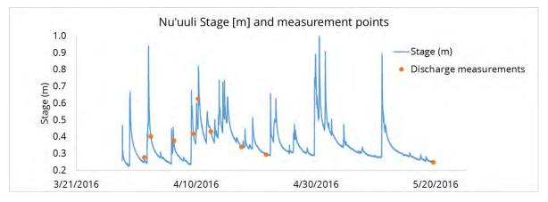
Figure 5. Example of stream stage and times where streamflow measurements were taken.
